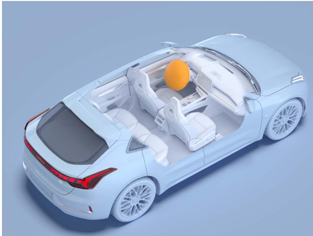
The front driver airbag is located in the center of the steering wheel. Its location is indicated by the AIRBAG marking on the steering wheel.
