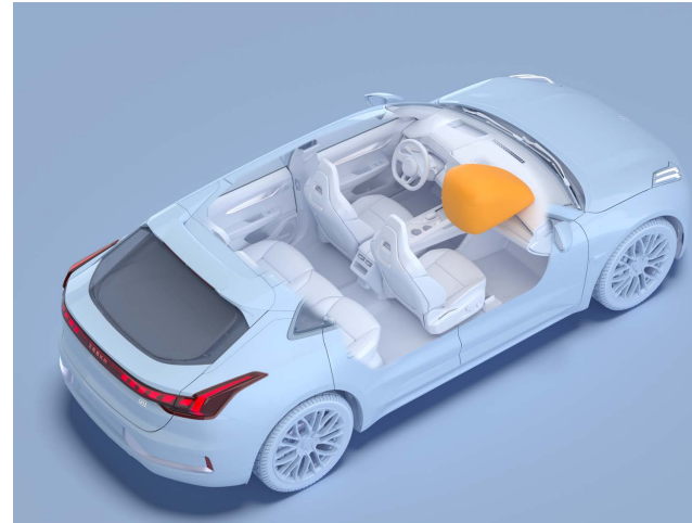
The front passenger airbag is located behind the panel above the glove compartment. Its location is indicated by the AIRBAG marking on that same panel.
